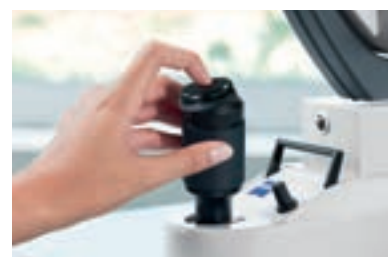
Navigating with fingertip precision: the electronic micromanipulator.
